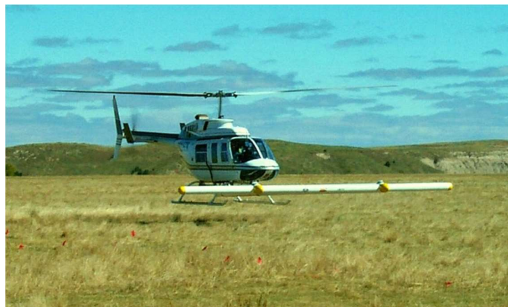
Figure 6-28: Example of an Airborne Geophysical System
