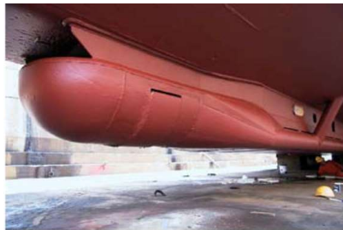
Figure 6-14: Example of an MBES Sensor
