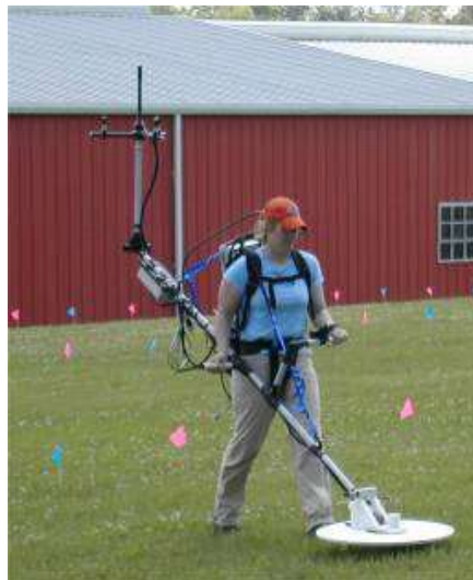
Figure 6-26: Example of a Man-Portable Geophysical System
