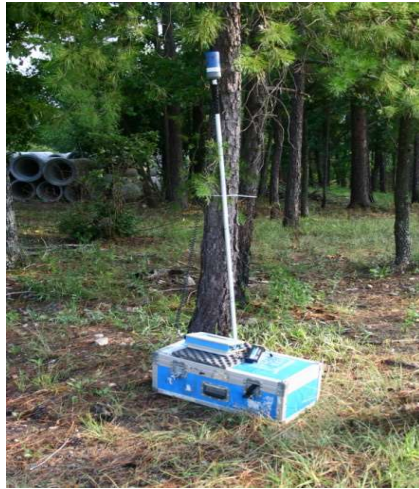
Figure 6-2: Geometrics G-856 Proton Precession Magnetometer
