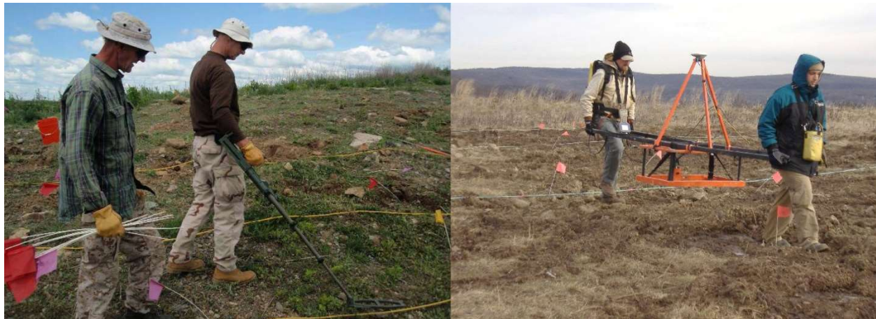
Figure 6-3: Vallon VMXC1 (left) and Geonics EM61-Mark 2 (MK2) (right) TDEMI Sensors
