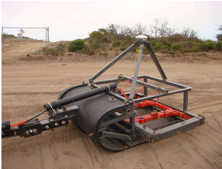
Figure 6-5: Example of a Towed TDEMI Array
