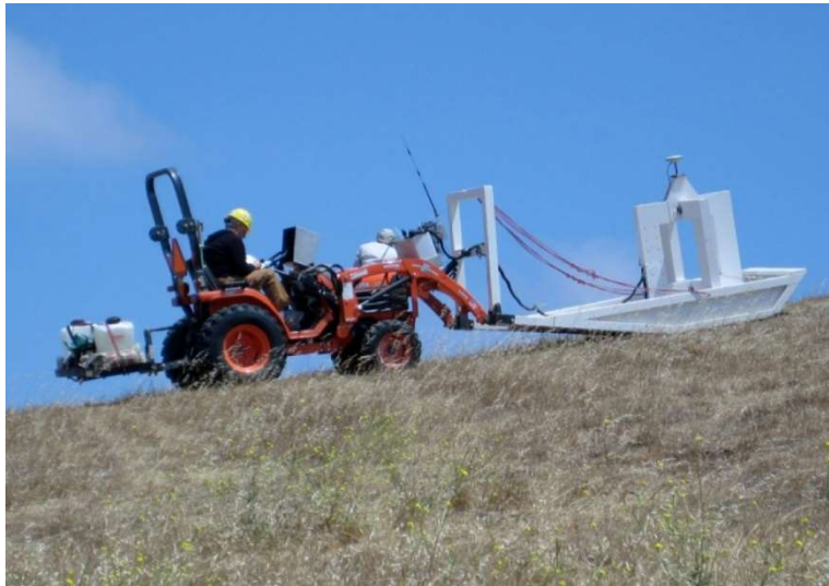
Figure 6-6: Geometrics MetalMapper™ Advanced EMI Sensor
